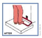
Redesigning the foot pedal reduces the force needed by the machine operator using it.
